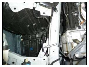
15. Position the mass air sensor wiring pigtail along the frame as shown.
