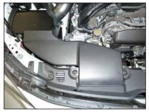
24. Reinstall the factory fresh air intake duct and secure with the factory hardware.
