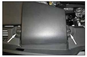
2. Remove the two clips that secure the fresh air intake duct and then remove the duct from the vehicle.
