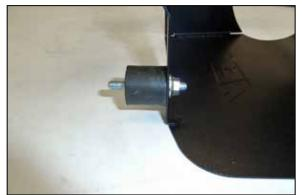
10. Install the provided rubber mounted stud onto the heat shield using the factory nut.
